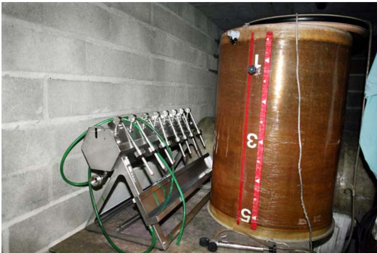
8-spout gravity bottle filler
